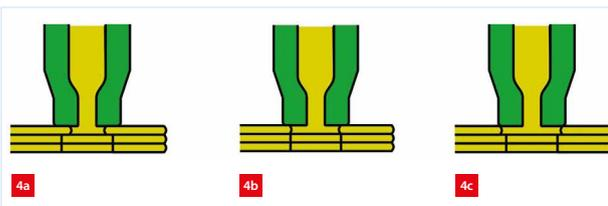
Flow of the molten polymer out of the nozzle of the print head under pressure control, as developed by Bond 3D, resulting in a homogeneous distribution of material regardless of the width of the gap that has to be filled.
