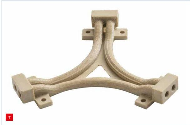
Printed manifold-like PEEK part (1.3 mm wall thickness) successfully subjected to a gas pressure test up to 100 bar.
